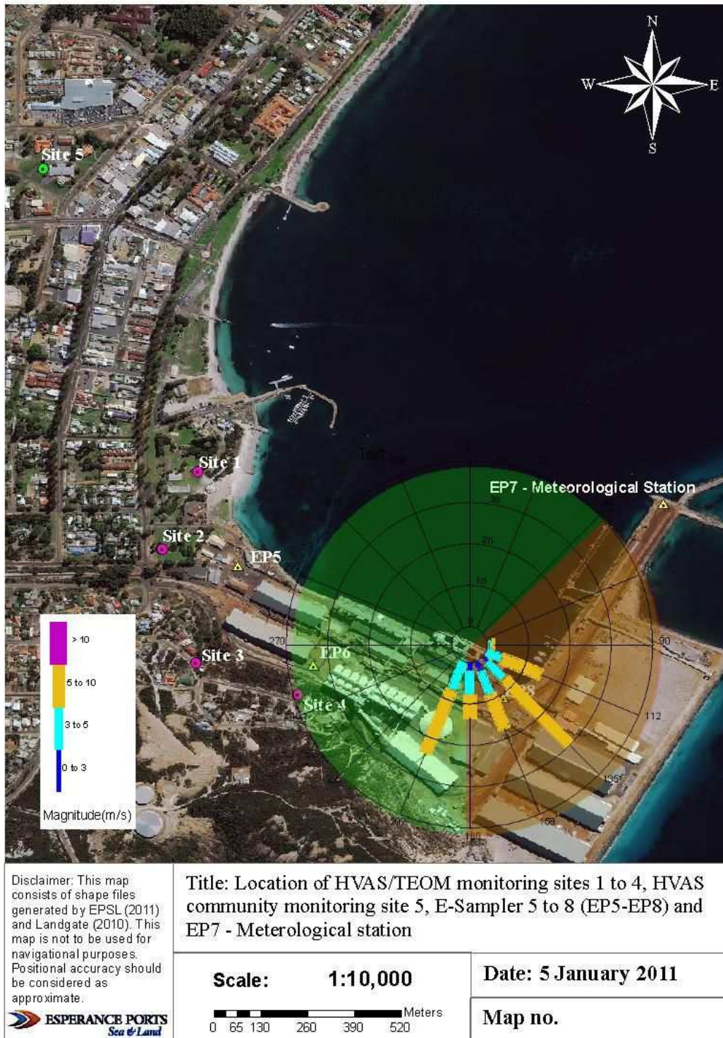
Figure 3: Wind arc zones, where 'red zone' is 45° to 180 ° and 'green zone' is 180 ° to 45° (EPSL, 2009a), showing loading wind rose data measured at the EP7 meteorological station from 0940 on 03/10/2011 to 1740 on 04/10/2011.
