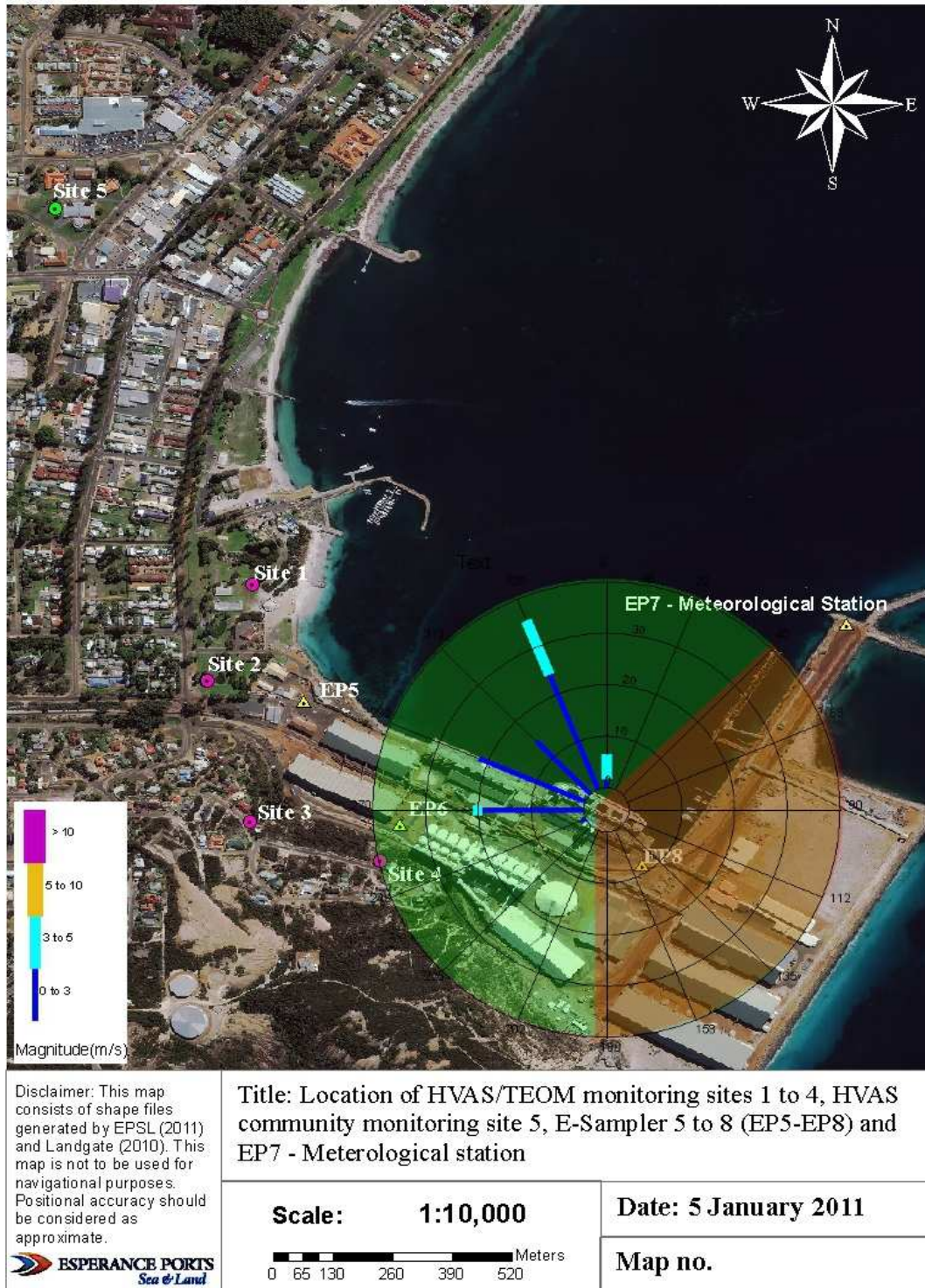
Figure 2. Wind arc zones defined in EPSL (2008), where 'red zone' is 45° to 180° and 'green zone' is 180° to 45°, showing loading wind rose data measured at the meteorological station adjacent to E-Sampler 7 from 1748 hours on 22/06/2011 to 0407 hours on 23/06/2011.
